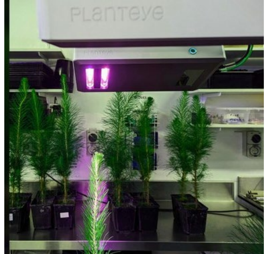
Phenospex PlantEye F600 – 3D multispectral scanner (proximal sensing, RGB + NIR)
